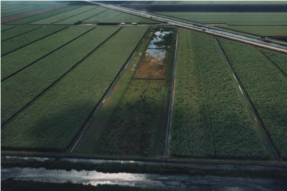
This is a phosphorus removal system for a sugar cane plantation in South Florida. It reduced phosphorus concentrations down to 20 parts per billion (ppb). Phosphorus concentrations in the drainage canals usually were in the 200 ppb range and regulatory discharge limits were 50 ppb.
