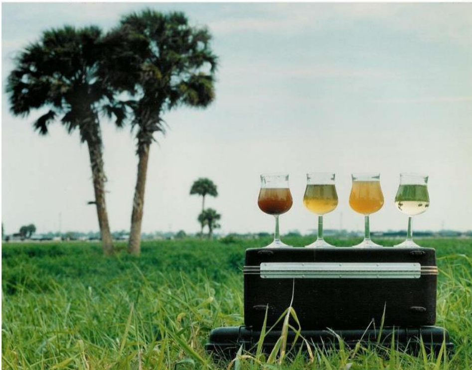
Water samples from the system, left to right. Barn washwater, pasture runoff influent to Bion system, bioreactor with microbes and phosphorus precipitate, final effluent. This system reduced barn and pasture runoff to less than one part per million of total phosphorus.
